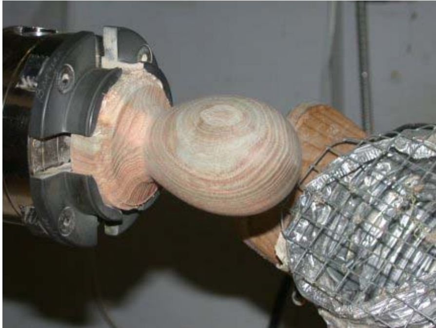
Stage 1 Turning completed prior to finishing
