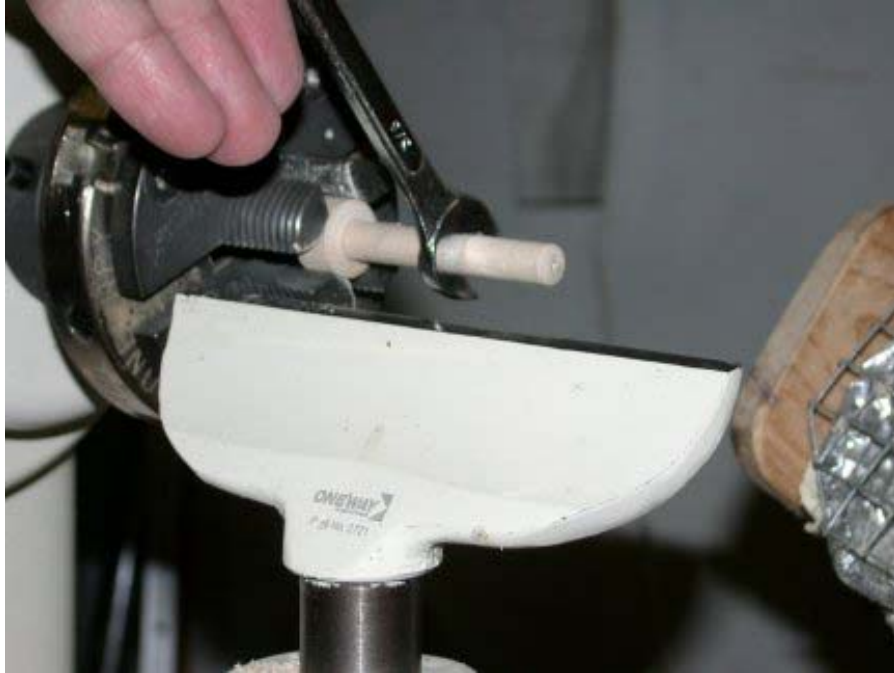
Sizing shaft of Knock-out Device with 3/8” Box End Wrench
