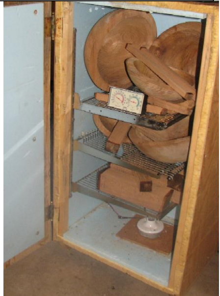
Photo 3 above The current load, made up of three large 14"-16" blanks, the core-outs and some spindle material. It has been in for three weeks and is pretty much near the end of its run. I have coated the endgrain on the larger bowls with wax emulsion on both inside and outside and have had almost zero problems with cracking. I have completed four loads to date and am immensely pleased with the overall results for the time and material investment.
