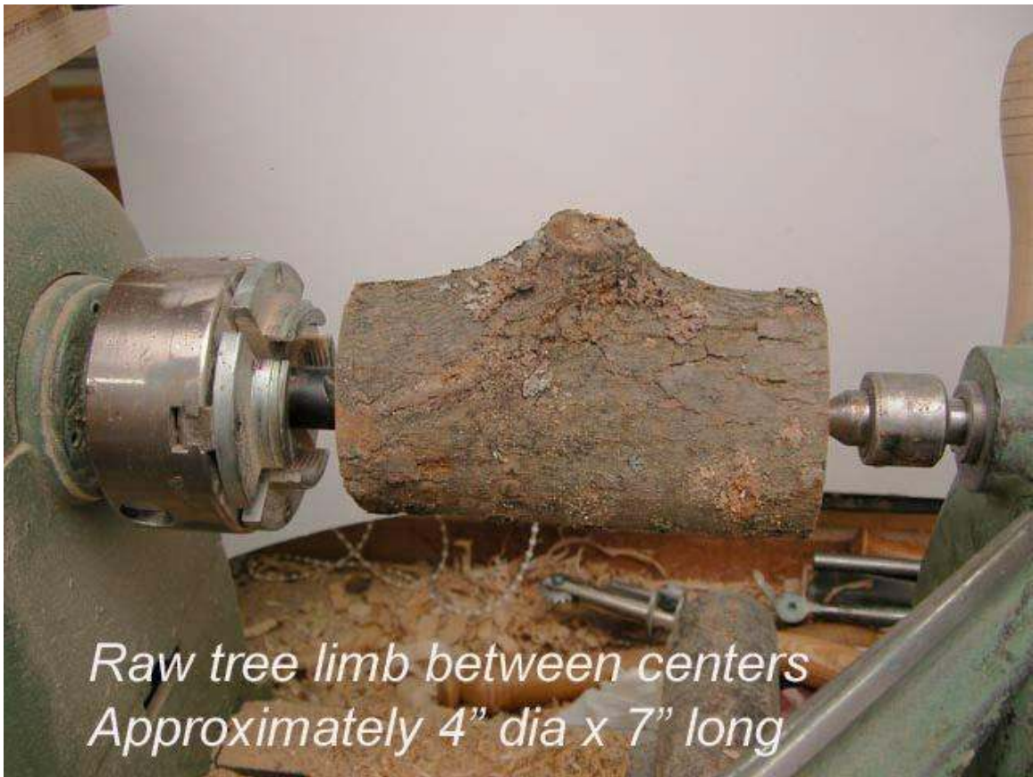
At the left is a removable drive spur, held with the #2 jaws in a Oneway Stronghold Chuck
